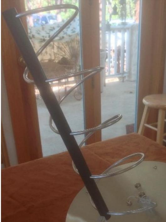
It has circular polarization. This allows it to communicate equally well regardless of the polarization from the other station. This makes it work well for satellite communication where polarization is constantly changing.
