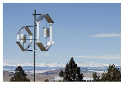
At the feed point the dipole or Isotron will resonate. This is when the Capacitance Reactance (XC) and Inductive reactance (XL) are equal (value in ohms). However, when this takes place, because the antenna is a radiator it will also develop a pure RESISTANCE (R) when resonant or Radiation Resistance. This R is dependent on the antennas grounding,
